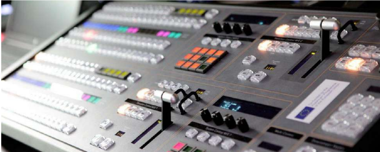
Figure 9 Broadcasting equipment - video mixer
